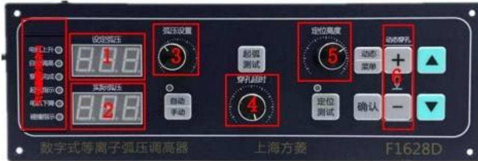
Figure 2. 4 F1628 Series Panel and Key Description
